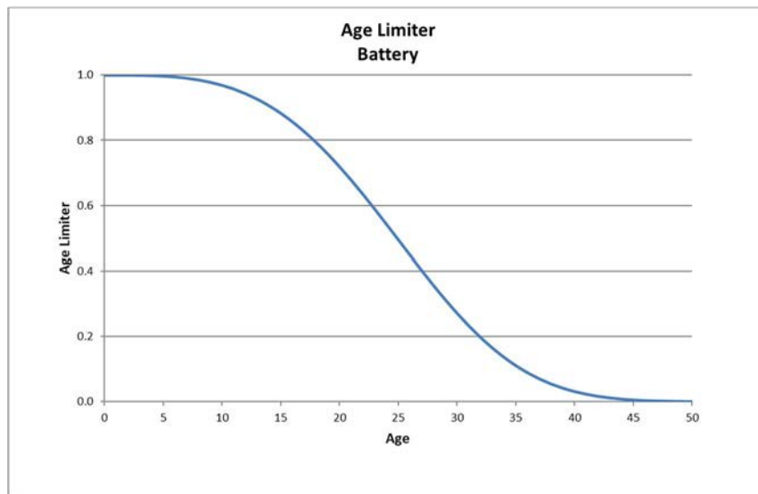
Figure A 15-2 Battery Banks Age Limiter
